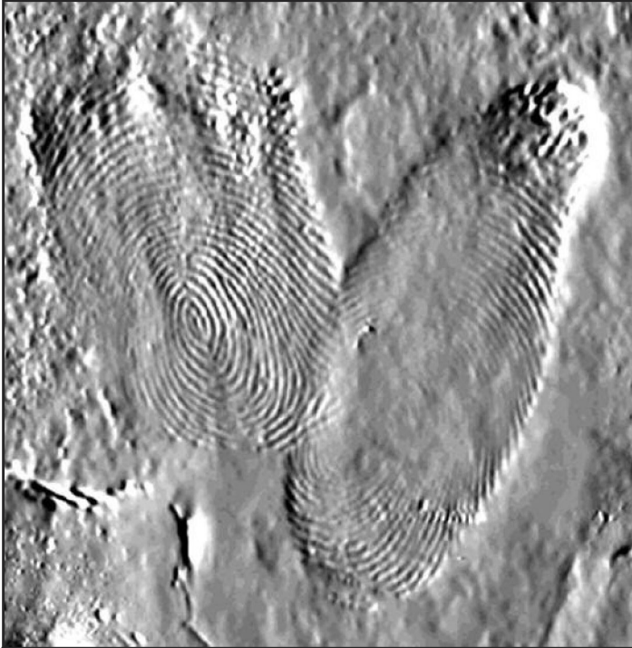
Figure 4: EPIC technology can be used to measure the electric charge pattern left behind by a finger when it touches a non-conductive surface.
